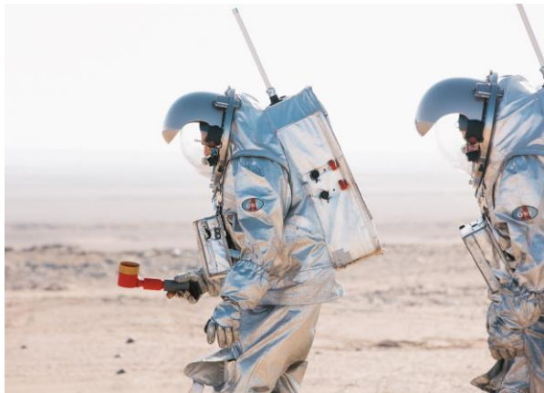
Figure 2: The ADAPT2Mars 3d-printing experiment deployed during the AMADEE-18 mission (red plastic and golden silica-coated steel printed soil sampling scoop)
