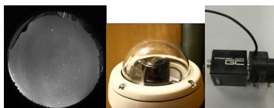
Figure 2: Bright meteor on night sky registered by all-sky camera installed in Kourvskaya observatory (Middle Ural) and view of Prosilica GC 1380 camera with objective.
