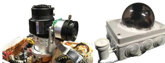
Figure 3: Internal and external view of Amateur station (QHY5LIIM camera and Computar 1.8-3.6mm 1.6 lens) operated by Raspberry Pi 2 Model B Rev 1.1. installed in Crimean observatory. It has 7m limiting magnitude and 110-degree field of view.
