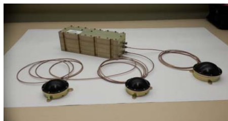
Figure 1: The LaRa transponder and its antennas (1 receiving antenna RX, 2 transmitting antennas TX).
